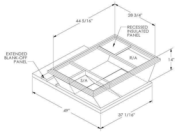
ONE PIECE WELDED CONSTRUCTION
