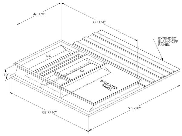
ONE PIECE WELDED CONSTRUCTION
