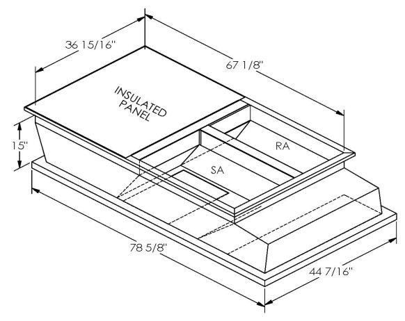
ONE PIECE WELDED CONSTRUCTION
