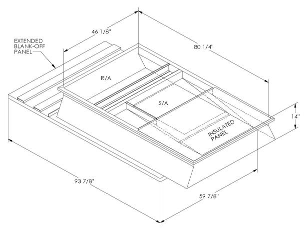
ONE PIECE WELDED CONSTRUCTION
