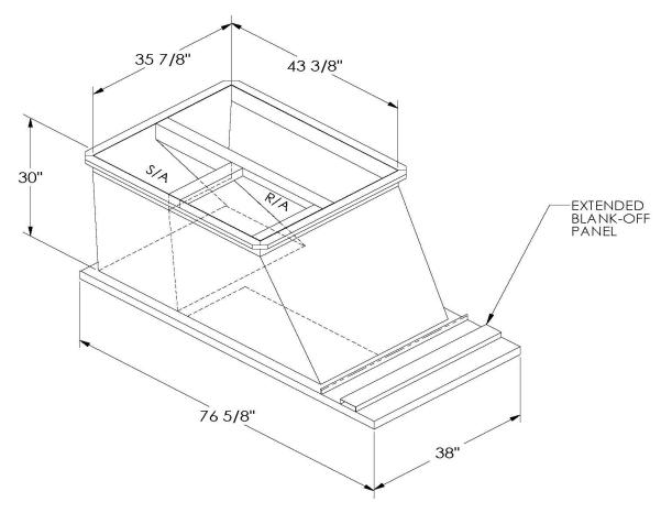
ONE PIECE WELDED CONSTRUCTION
