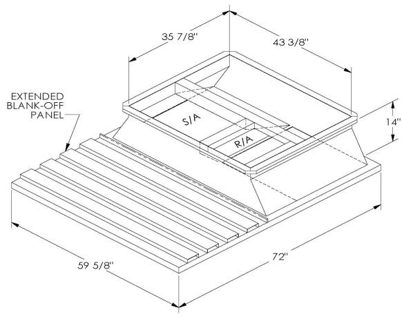
ONE PIECE WELDED CONSTRUCTION
