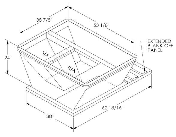
ONE PIECE WELDED CONSTRUCTION
