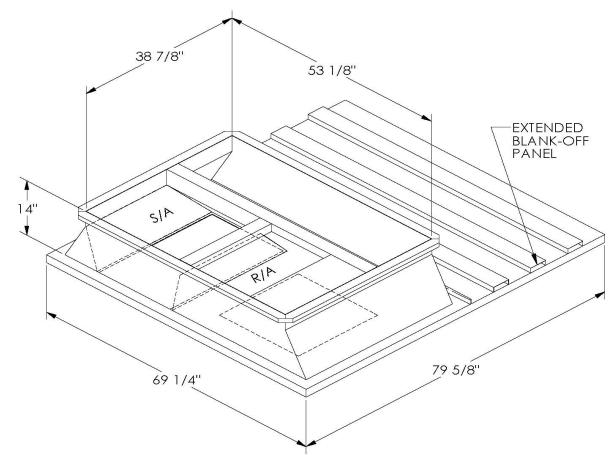
ONE PIECE WELDED CONSTRUCTION
