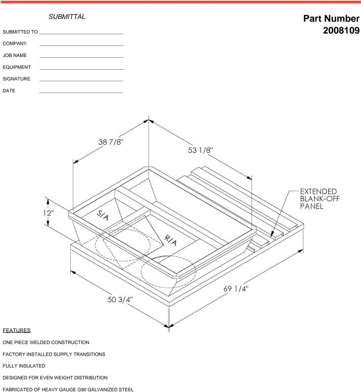
ALL WELDS SPRAYED WITH GALVANIZING COMPOUND
