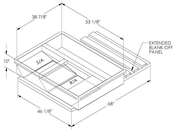
ONE PIECE WELDED CONSTRUCTION
