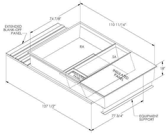
ONE PIECE WELDED CONSTRUCTION
