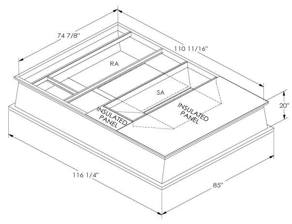
ONE PIECE WELDED CONSTRUCTION
