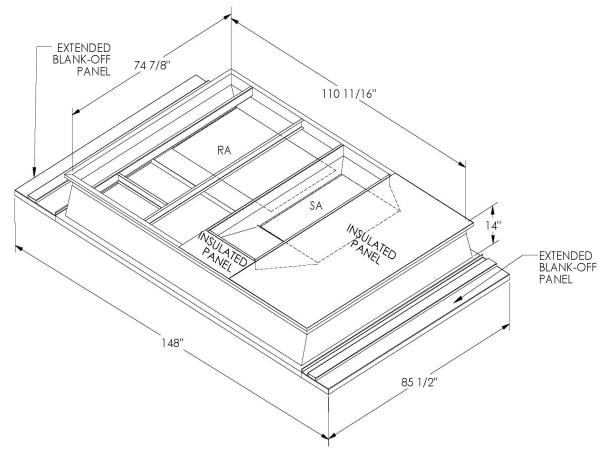
ONE PIECE WELDED CONSTRUCTION
