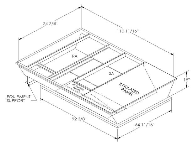
ONE PIECE WELDED CONSTRUCTION
