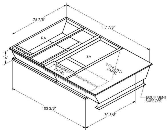
ONE PIECE WELDED CONSTRUCTION
