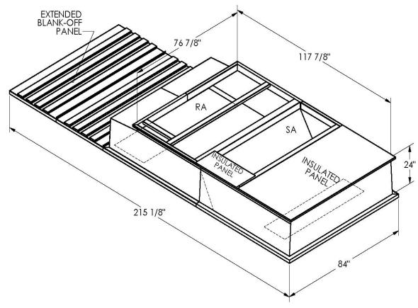
ONE PIECE WELDED CONSTRUCTION
