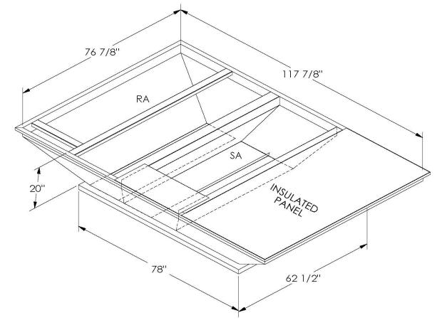
ONE PIECE WELDED CONSTRUCTION
