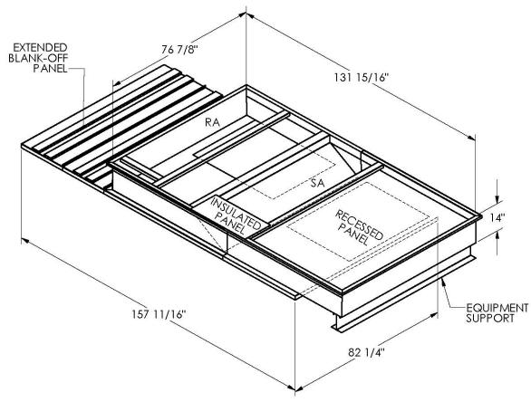
ONE PIECE WELDED CONSTRUCTION
