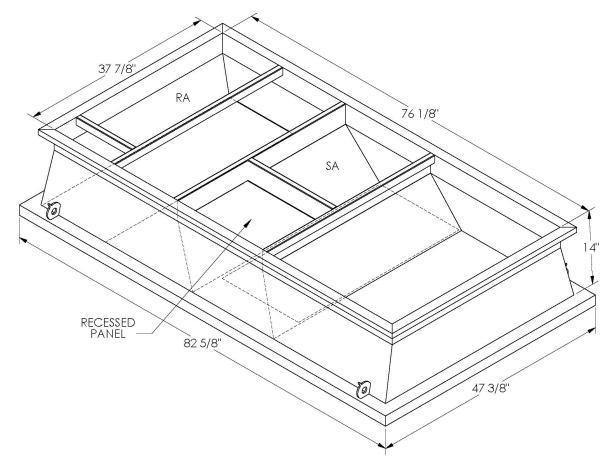
ONE PIECE WELDED CONSTRUCTION
