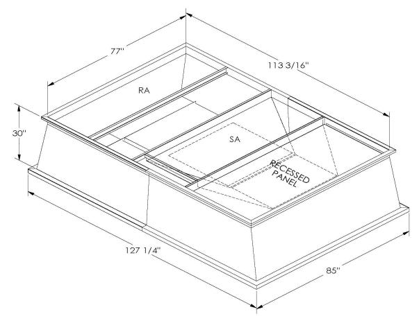
ONE PIECE WELDED CONSTRUCTION
