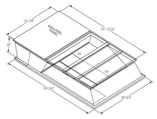
ONE PIECE WELDED CONSTRUCTION
