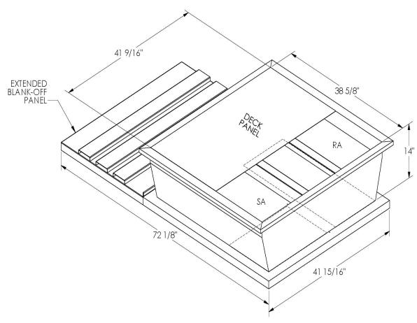
ONE PIECE WELDED CONSTRUCTION
