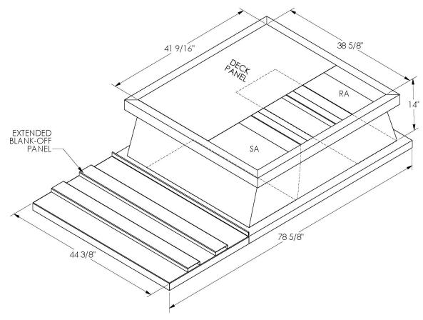
ONE PIECE WELDED CONSTRUCTION
