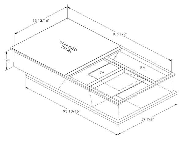
ONE PIECE WELDED CONSTRUCTION
