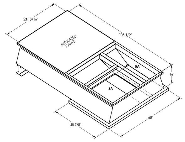
ONE PIECE WELDED CONSTRUCTION
