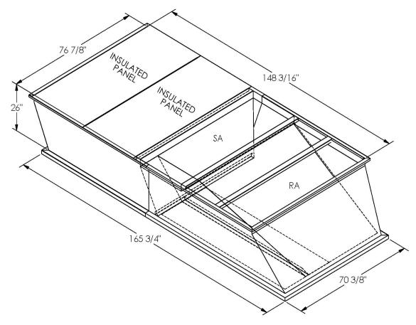
ONE PIECE WELDED CONSTRUCTION
