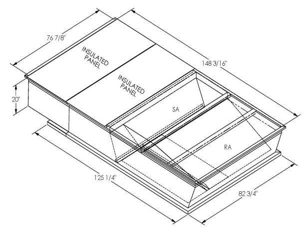
ONE PIECE WELDED CONSTRUCTION
