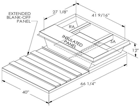
ONE PIECE WELDED CONSTRUCTION
