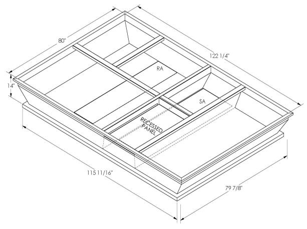
ONE PIECE WELDED CONSTRUCTION
