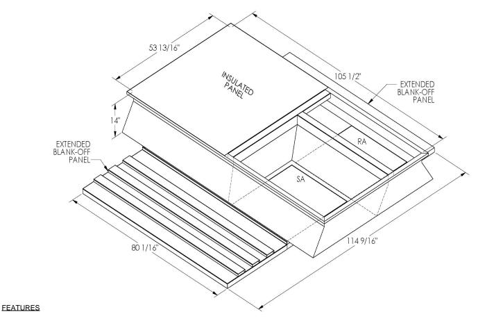
ONE PIECE WELDED CONSTRUCTION
