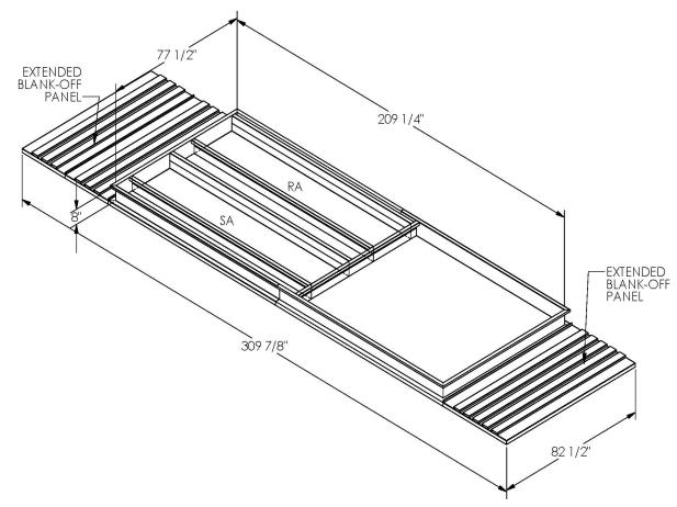
ONE PIECE WELDED CONSTRUCTION
