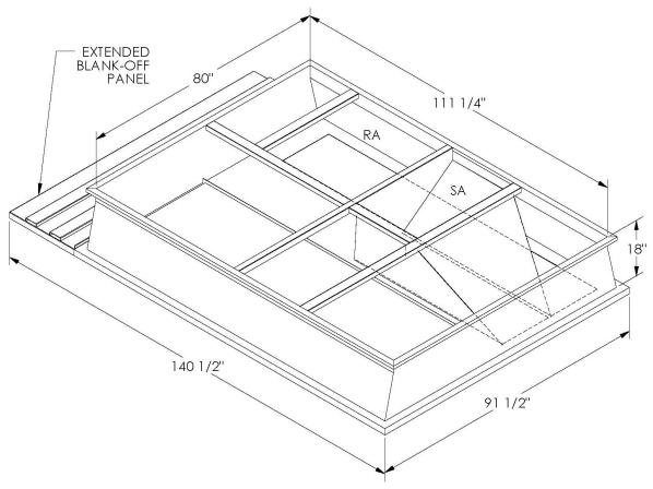
ONE PIECE WELDED CONSTRUCTION
