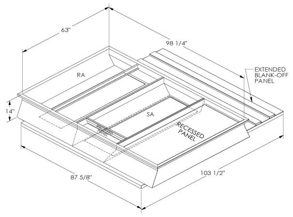
ONE PIECE WELDED CONSTRUCTION
