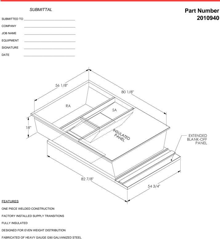
ALL WELDS SPRAYED WITH GALVANIZING COMPOUND
