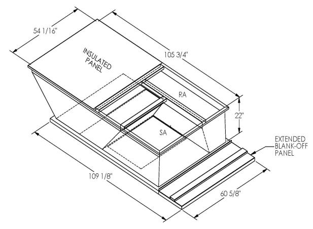
ONE PIECE WELDED CONSTRUCTION
