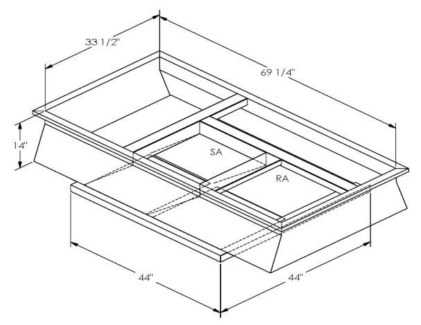
ONE PIECE WELDED CONSTRUCTION
